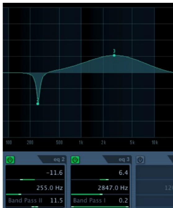
Figure 8: 2 EQs in cubase. Note the cut frequency represented by the point in the curve, and the width of the curve, which corresponds to the Q of the filter.
